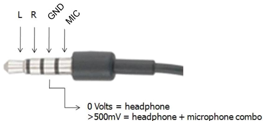
Plug insertion is reported on the headphone port using the switch integrated into the jack.
