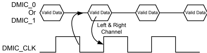
Figure 6. Stereo Digital Microphone Configuration
