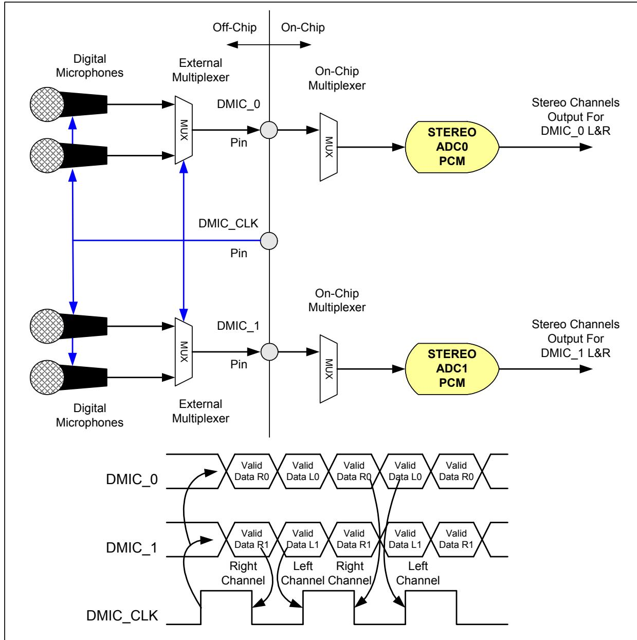
*Note: Some Digital Microphone Implementations support data on either edge, in this case the external multiplexer is not required.*
