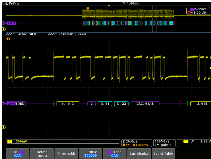
Color-coded display of a CAN bus, showing Start, DLC, Data, CRC, and Stop components of the serial signal.
