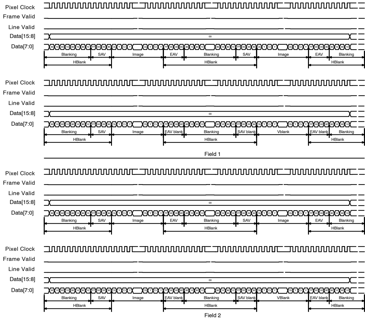
Figure 18. Typical CCIR656 Output
