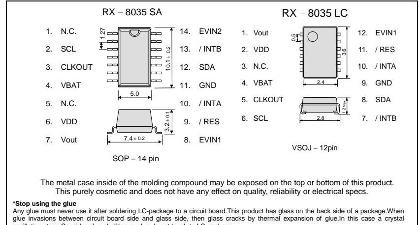
The metal case inside of the molding compound may be exposed on the top or bottom of this product.
