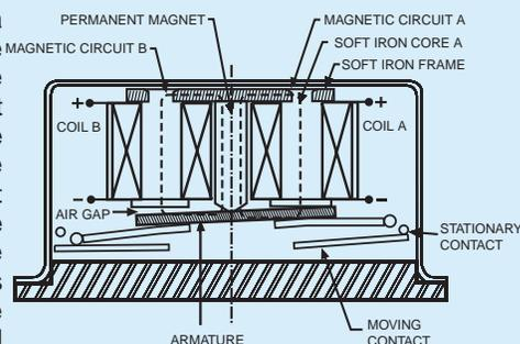
When latching relays are installed in equipment, the latch and reset coils should not be pulsed simultaneously. Coils should not be pulsed with less than rated coil voltage and the pulse width should be a minimum of three times the specified operate time of the relay. If these conditions are not followed, it is possible for the relay to be in the magnetic neutral position.
