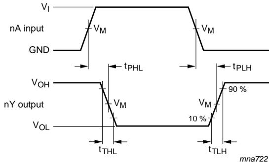
$V_M = 0.5 \times V_{CC}$ ;  $V_I = \text{GND to } V_{CC}$ .
