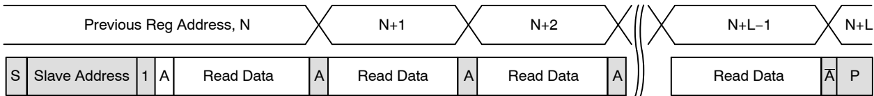
Figure 37. Sequential READ, Start from Current Location
