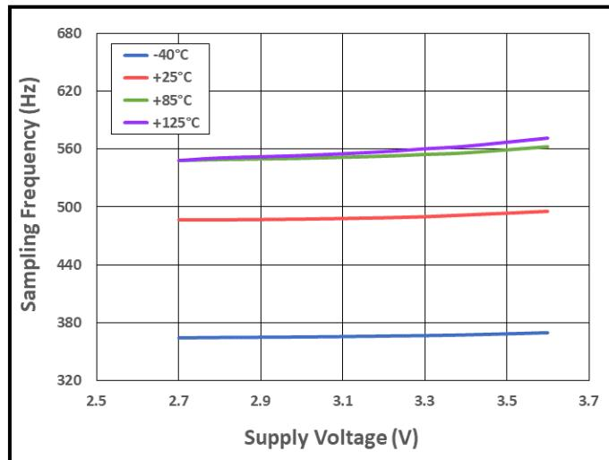
**Figure 6.** Sampling Frequency vs. Supply Voltage vs. Temperature
