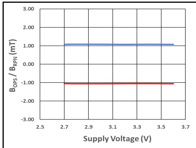
**Figure 7.**  $B_{OPS}$  (Blue) and  $B_{RPN}$  (Red) vs. Supply Voltage at  $+25^\circ\text{C}$
