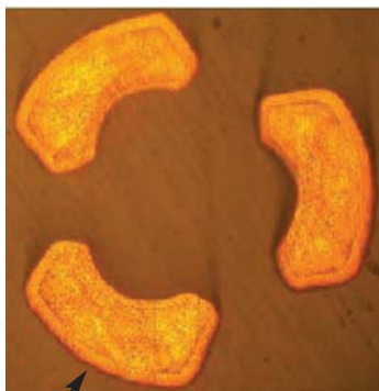
Au/Ni Barrier (Uniform plating thickness)
