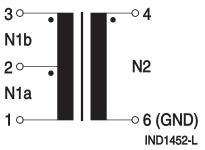
Recommendation: Connect pin 6 on PCB to GND
