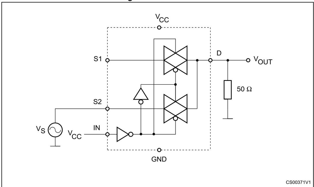
Figure 5. OFF leakage
