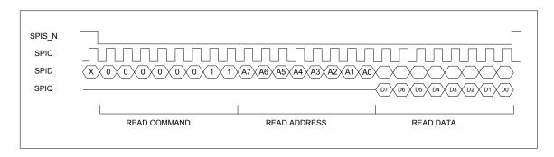
Figure 11. SPI Read Data Cycle
