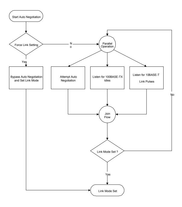
Figure 3. Auto-Negotiation and Parallel Operation
