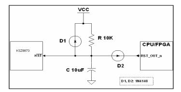
Figure 31. Recommended Reset Circuit for interfacing with CPU/FPGA Reset Output
