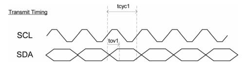
Figure 16. EEPROM Interface Output Timing Diagram
