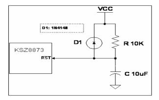
Figure 30. Recommended Reset Circuit
