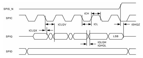
Figure 26. SPI Output Timing
