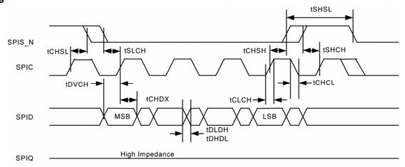
Figure 25. SPI Input Timing
