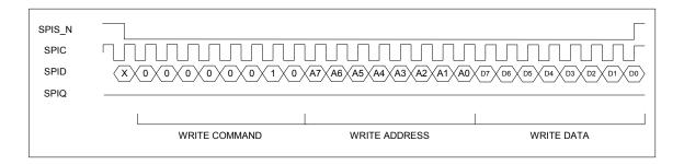
Figure 10. SPI Write Data Cycle
