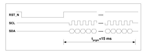
Figure 9. EEPROM Configuration Timing Diagram
