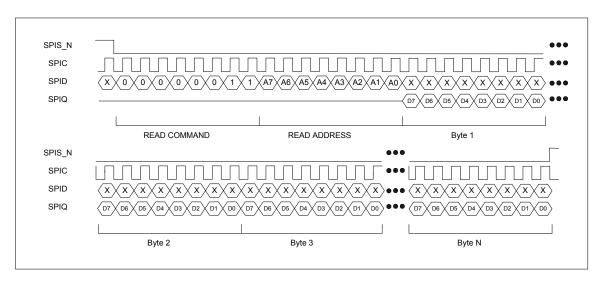
Figure 13. SPI Multiple Read
