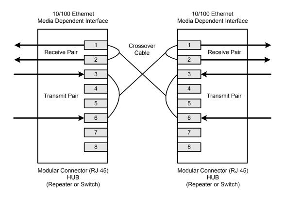
Figure 2. Typical Crossover Cable Connection
