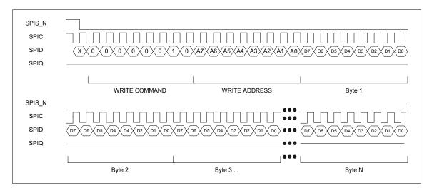
Figure 12. SPI Multiple Write
