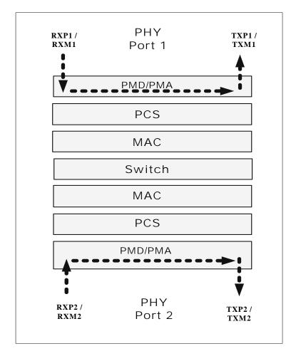
Figure 14. Near-end (Remote) Loopback Path
