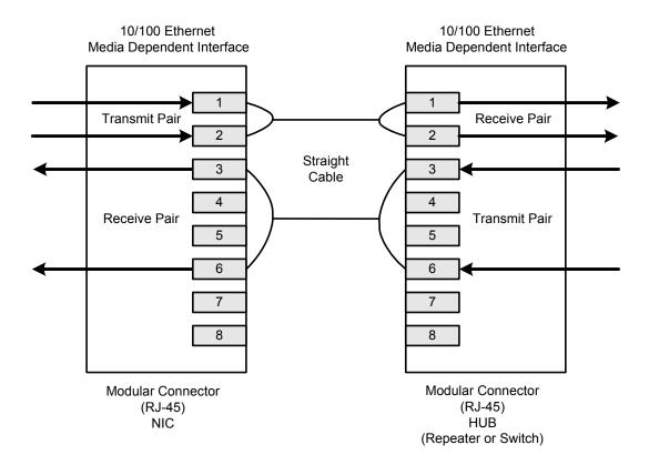
Figure 1. Typical Straight Cable Connection
