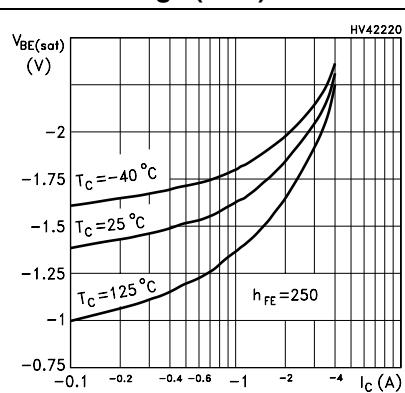
**Figure 10. Base-emitter on voltage (NPN)**
