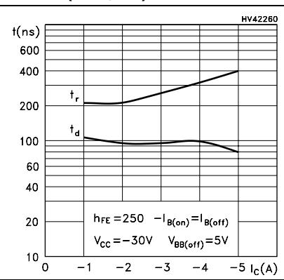
Figure 14. Resistive load switching time (NPN, off)    Figure 15. Resistive load switching time (PNP, off)
