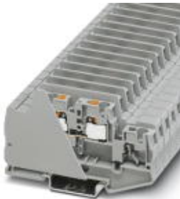
Feed-through terminal block, Connection method: Push-in connection, Cross section: 0.2 mm 2 - 6 mm 2 , AWG: 24 - 10, Width: 8.2 mm, Color: gray, Mounting type: NS 35/7,5, NS 35/15
