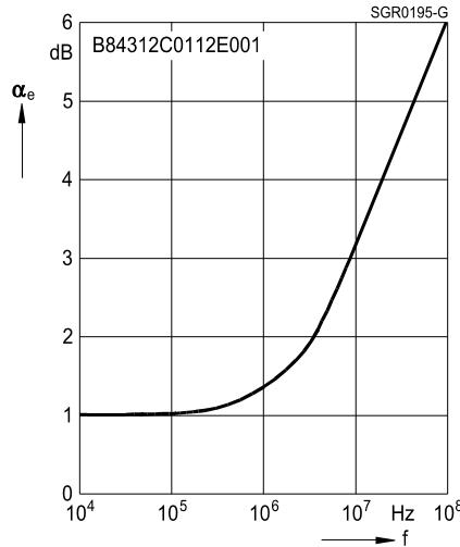
Insertion loss  $\alpha_e$  in stopband (typical)
