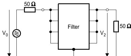
$$\alpha_e = 20 \lg \frac{V_0}{2 \cdot V_2} [\text{dB}]$$
