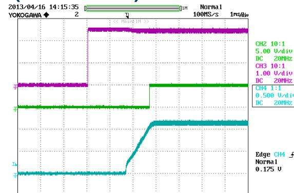
**Figure 14:** Turn on delay time at 12Vin, 1.2V/40A out (4mS/div)
