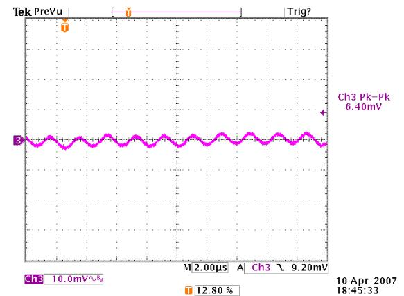
**Figure 11:** Output ripple & noise at 12Vin, 3.3V/40A out
