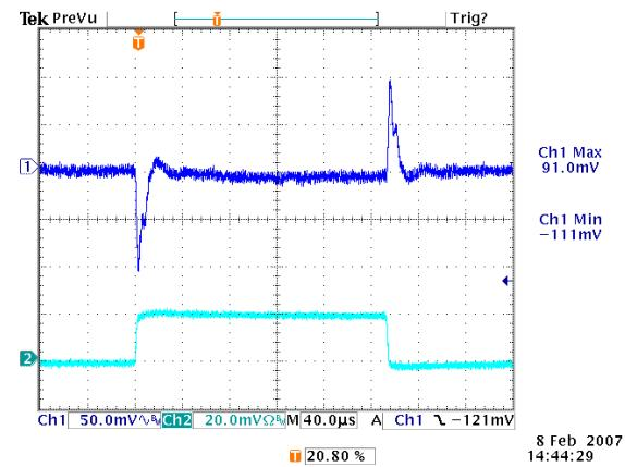
**Figure 22:** Transient Response at 12Vin, 2.5V/40A out (40uS/div)
