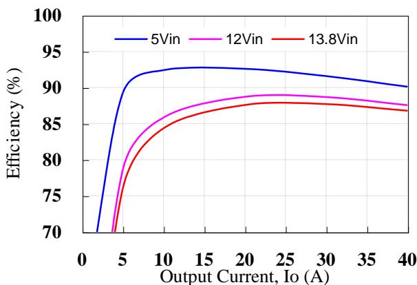
**Figure 3:** Converter efficiency vs. output current
