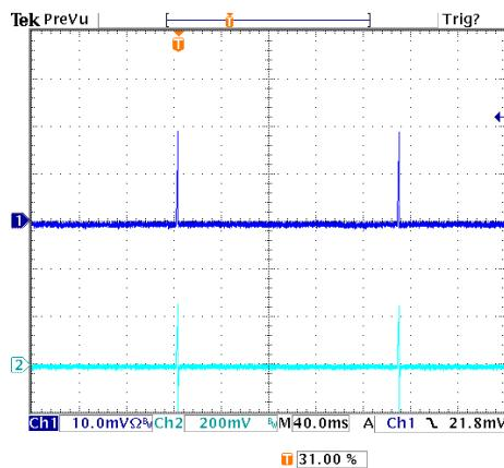
**Figure 25:** Short Circuit Protection at 12Vin, 0.9V out (40mS/div),
