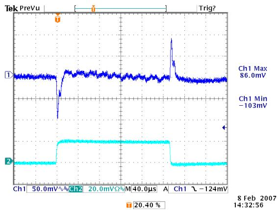
**Figure 21:** Transient Response at 12Vin, 1.8V/40A out (40uS/div)
