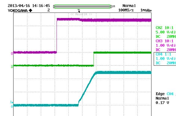
**Figure 16:** Turn on delay time at 12Vin, 2.5V/40A out (4mS/div)
