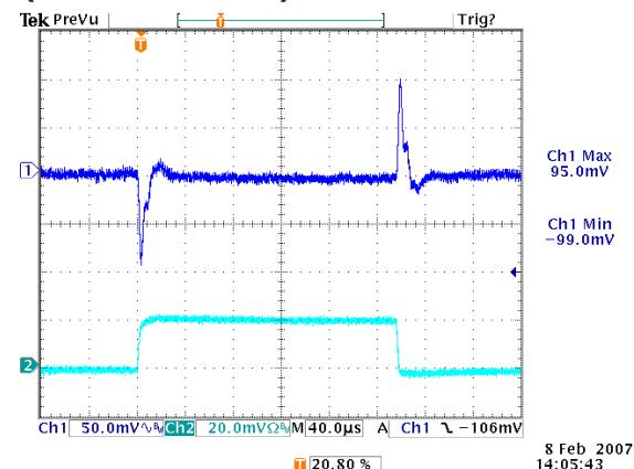
**Figure 20:** Transient Response at 12Vin, 1.2V/40A out (40uS/div)
