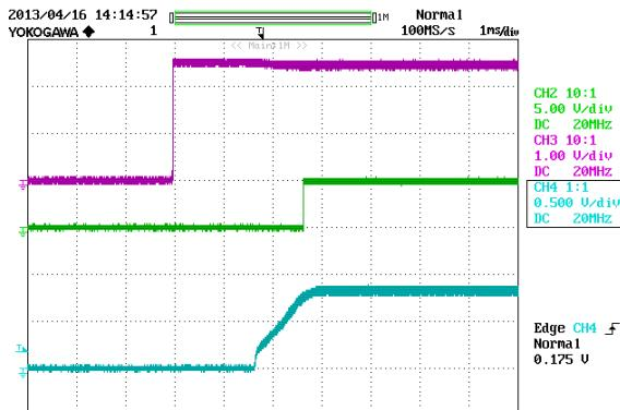
**Figure 13:** Turn on delay time at 12Vin, 0.9V/40A out (4mS/div)
