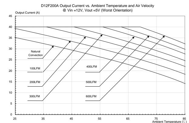
**Figure 38:** Output current vs. ambient temperature and air velocity @ $Vin=12V$ ,  $Vout=5.0V$  (Airflow from Pin1 to Pin11)
