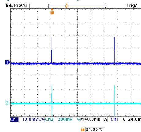
**Figure 26:** Short Circuit Protection at 12Vin, 1.2V out (40mS/div),
