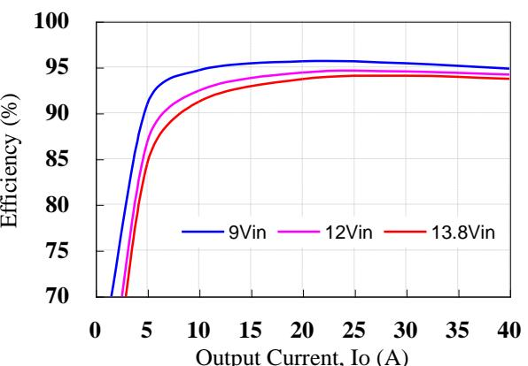
**Figure 6:** Converter efficiency vs. output current
