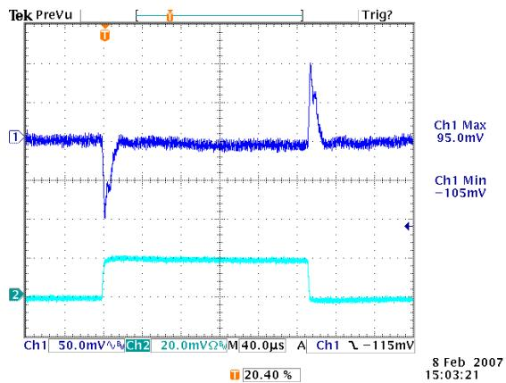
**Figure 23:** Transient Response at 12Vin, 3.3V/40A out (40uS/div)
