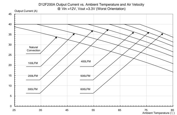
**Figure 39:** Output current vs. ambient temperature and air velocity@  $Vin=12V$ ,  $Vout=3.3V$  (Worst Orientation)
