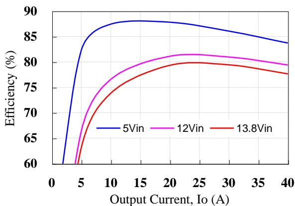
**Figure 1:** Converter efficiency vs. output current
