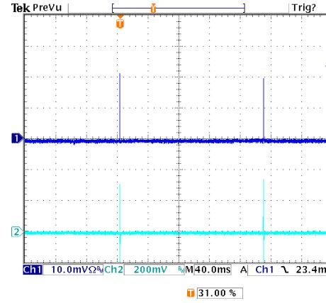
**Figure 28:** Short Circuit Protection at 12Vin, 2.5V out (40mS/div),
