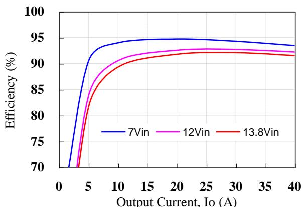
**Figure 5:** Converter efficiency vs. output current
