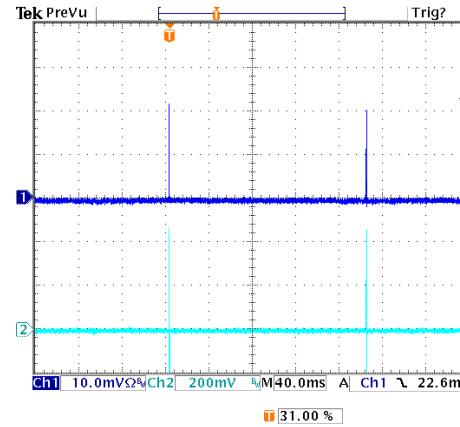
**Figure 30:** Short Circuit Protection at 12Vin, 5.0V out (40mS/div),
