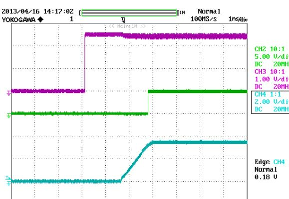
**Figure 17:** Turn on delay time at 12Vin, 3.3V/40A out (4mS/div)
