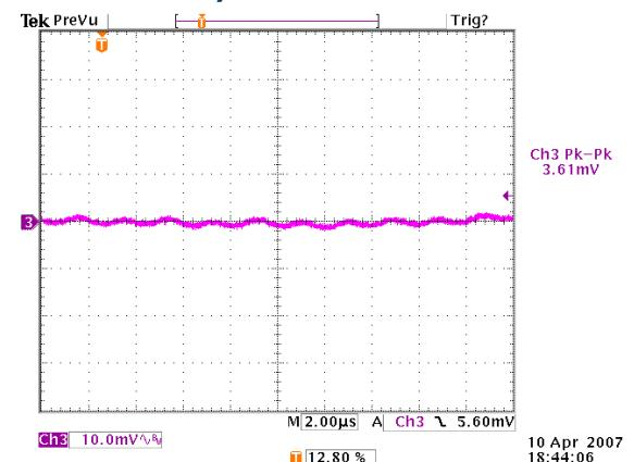
**Figure 7:** Output ripple & noise at 12Vin, 0.9V/40A out
