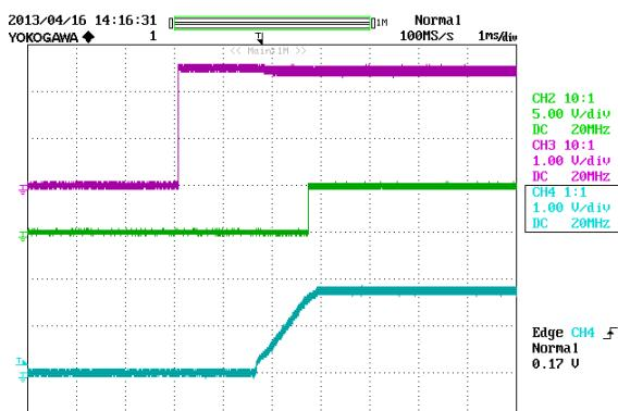
**Figure 15:** Turn on delay time at 12Vin, 1.8V/40A out (4mS/div)
