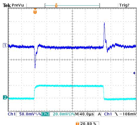
**Figure 19:** Transient Response at 12Vin, 0.9V/40A out (40uS/div)
