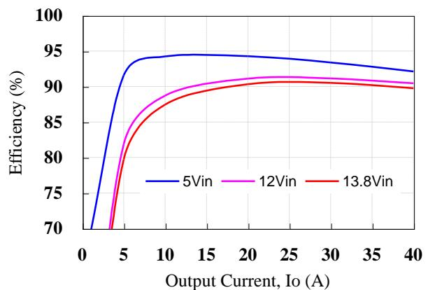
**Figure 4:** Converter efficiency vs. output current
