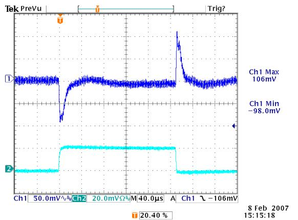
**Figure 24:** Transient Response at 12Vin, 5.0V/40A out (40uS/div)
