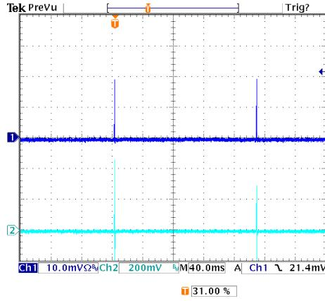
**Figure 27:** Short Circuit Protection at 12Vin, 1.8V out (40mS/div),
