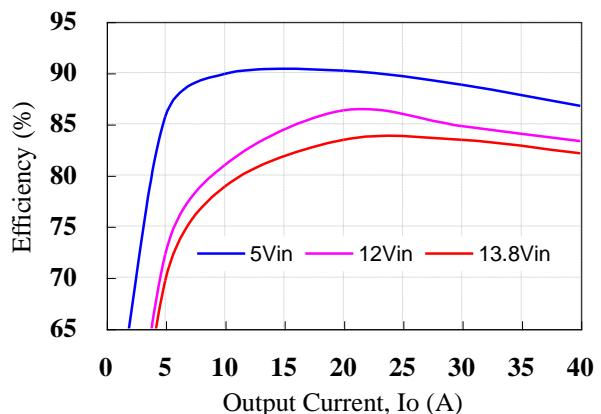
**Figure 2:** Converter efficiency vs. output current
