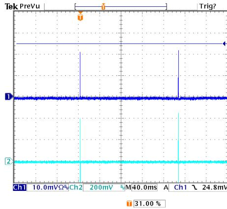
**Figure 29:** Short Circuit Protection at 12Vin, 3.3V out (40mS/div),
