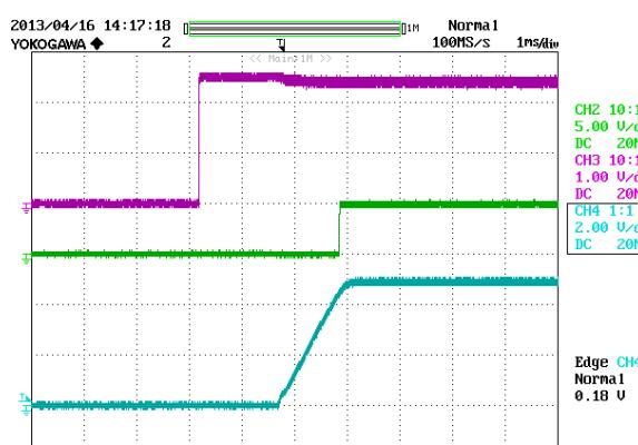
**Figure 18:** Turn on delay time at 12Vin, 5.0V/40A out (4mS/div)
