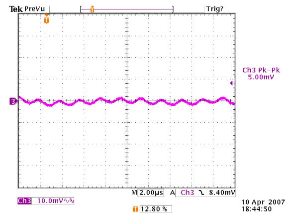
**Figure 9:** Output ripple & noise at 12Vin, 1.8V/40A out
