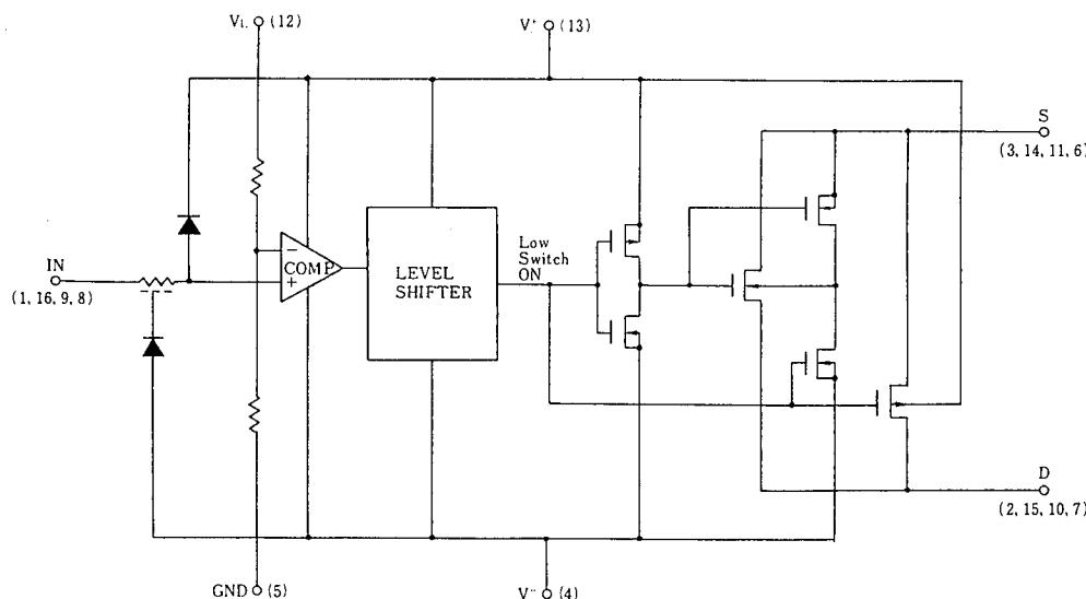
\* Logic input threshold voltage  $V_{TH}$  is about  $V_L \times 0.384(V)$ .
