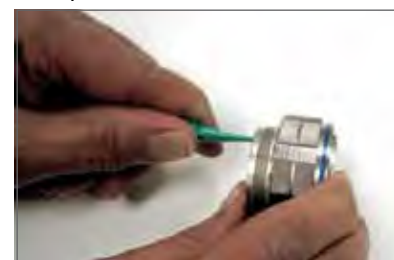
Plastic tool with contact in proper position.
