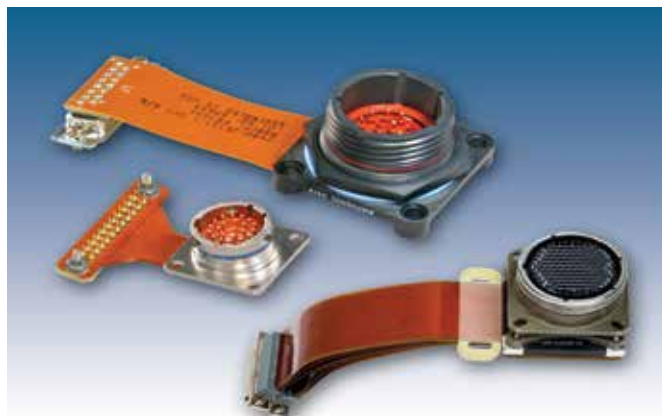
Flex Termination for Attachment to PC Boards
