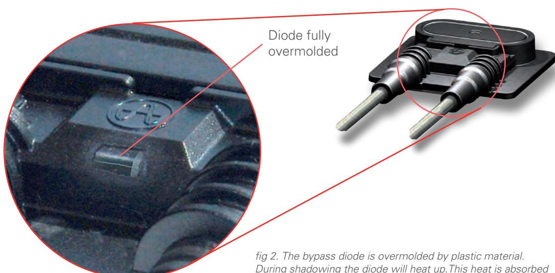
fig 2. The bypass diode is overmolded by plastic material. During shadowing the diode will heat up. This heat is absorbed and eliminated. The plastic material has a 30 times higher heat conductivity than air.
