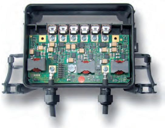
Silicon is a Semiconductor. It is conductive under light. It becomes non conductive when shadowed. In the case of partial shadowing on a PV panel, the affected cell area must be controlled by the Junction Box
