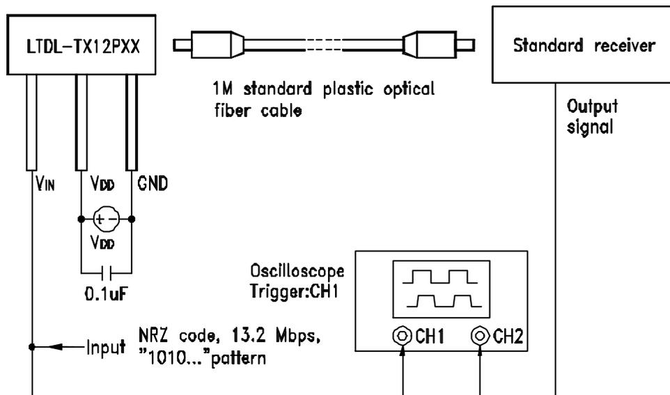
**Rise and Fall Times and Pulse Width Distortion**
