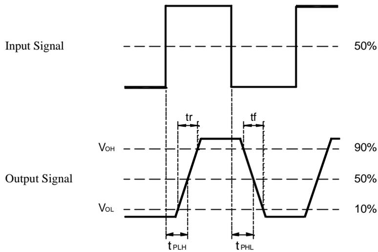
*Pulse Width Distortion =  $\Delta tw = t_{PHL} - t_{PLH}$*
