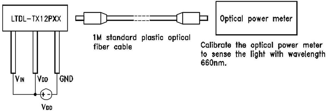
**\*2 Measuring method of pulse response and jitter**
