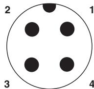
Figure 3 Pin assignment of the I/O link interface
