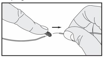
If the exposed metal ends of some of the wires break off due to great use, you should just simply remove 3/8" if the insulation from the wire of the broken end and then simply twist the strands together. To remove the installation you can use either a wirestripper tool or a simple penknife. Be extremely careful when doing this because penknives are remarkably sharp.
