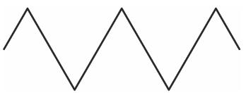
The shape of this wave results from the slow charging of the  $0.1\mu F$  capacitor through the control and the  $100k\Omega$  resistor, and the capacitor's discharge through the PNP and NPN transistors.
