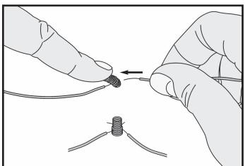
Only insert the exposed or shiny part of the wire into the spring terminal. The electrical connection will not be made if the plastic part of the wire is inserted into the terminal. Removing the wire from the spring terminals is simply just bending each terminal and then pulling the wires out of it.
