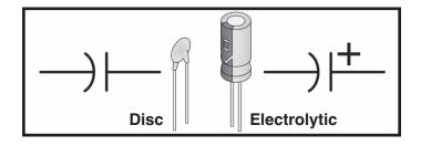
*Disc* - Unlike the electrolytic above, these capacitors have no polarity and can be connected in either way.
