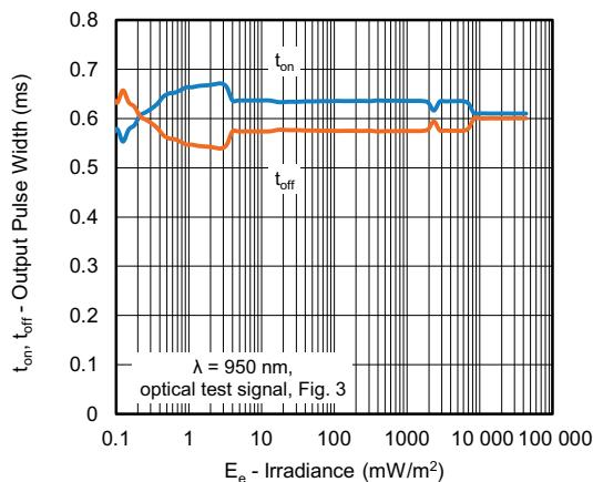
Fig. 4 - Pulse-Width vs. Irradiance in Dark Ambient
