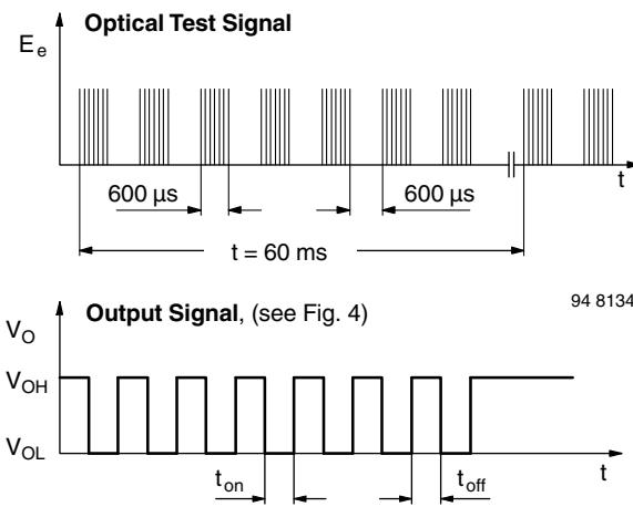
Fig. 3 - Test Signal
