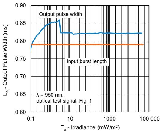
Fig. 2 - Pulse-Width vs. Irradiance in Dark Ambient
