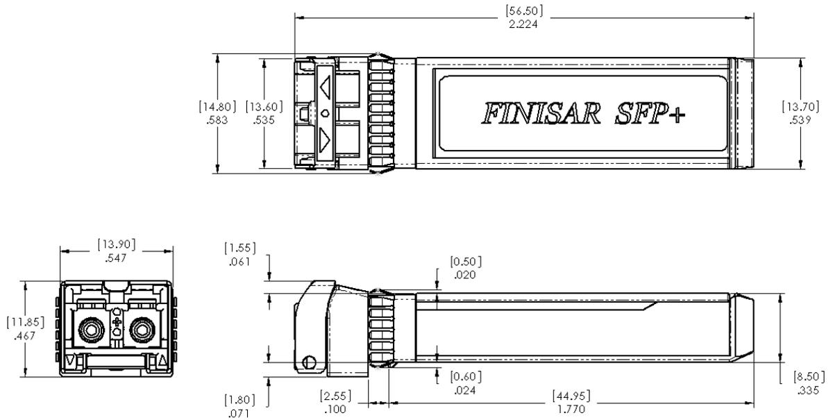
**Figure 3. FTLX8571D3BCL Mechanical Dimensions.**
