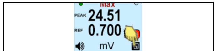
Figure 34. Using the Data Storage button
