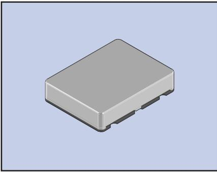
The VC-TXO-39SMX is a VC (Voltage Controlled) TCXO (Temperature Compensated Crystal Oscillator) featuring very tight stability over a wide temperature range. The small SMD ceramic package measures 11.4 x 9.6 x 2.3 mm. The voltage control has a tuning range of  $\pm 12$  ppm typical. The low profile package is ideal for wireless communications applications.
