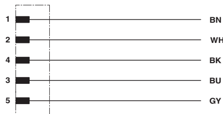
Contact assignment of the M12 plug
