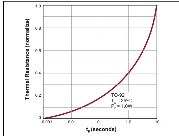
**FIGURE 2-12:** Thermal Response Characteristics.
