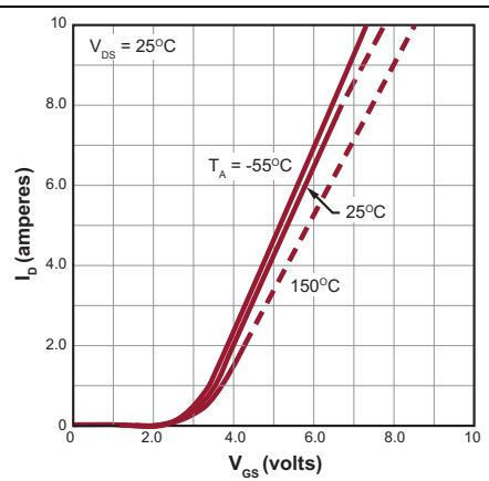
**FIGURE 2-2:** Transfer Characteristics.
