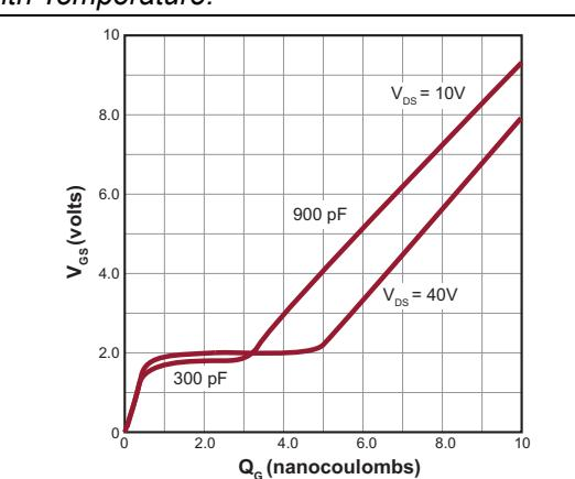
**FIGURE 2-6:** Gate Drive Dynamic Characteristics.
