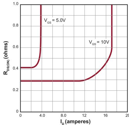
**FIGURE 2-4:** On-resistance vs. Drain Current.
