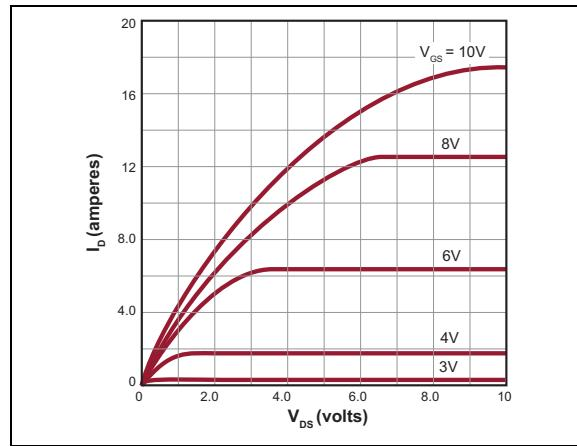
**FIGURE 2-10:** Saturation Characteristics.
