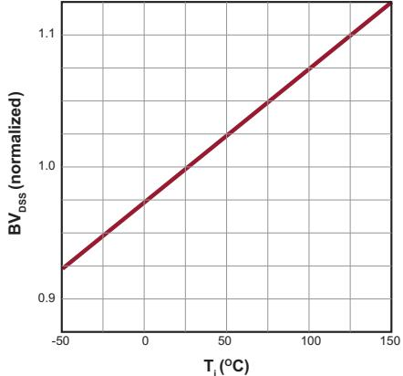
**FIGURE 2-1:**  $BV_{DSS}$  Variation with Temperature.
