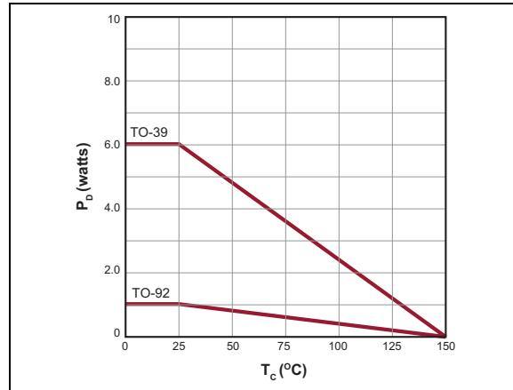
**FIGURE 2-11:** Power Dissipation vs. Case Temperature.
