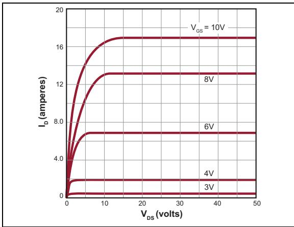
**FIGURE 2-7:** Output Characteristics.
