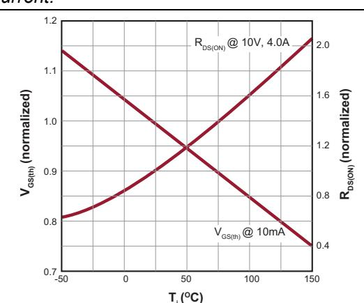
**FIGURE 2-5:**  $V_{GS}$  and  $R_{VDS}$  Variation with Temperature.
