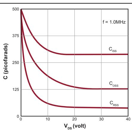
**FIGURE 2-3:** Capacitance vs. Drain-to-source Voltage.
