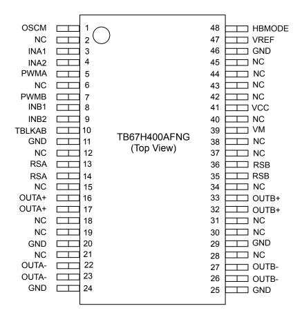
Note: Please connect the HTSSOP exposed pad to the PCB ground pattern.
