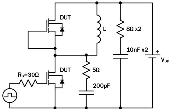
**Figure 13. Switching Time Test Circuit**
