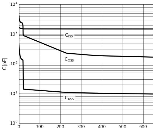
**Figure 5. Typical Capacitance**
