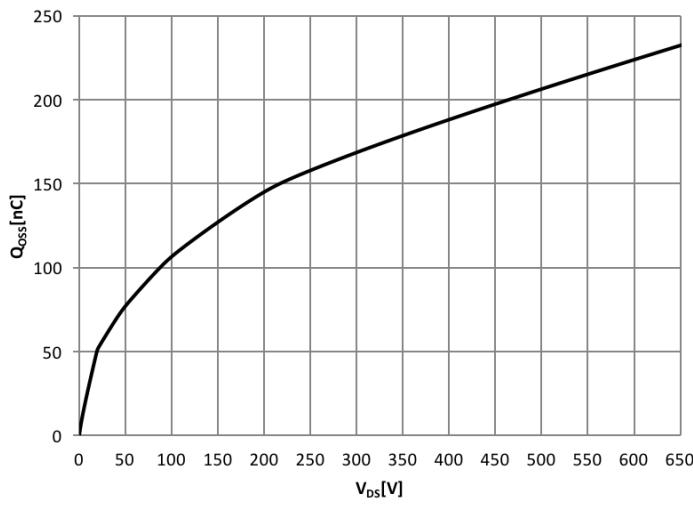
**Figure 7. Typical  $Q_{\text{oss}}$**
