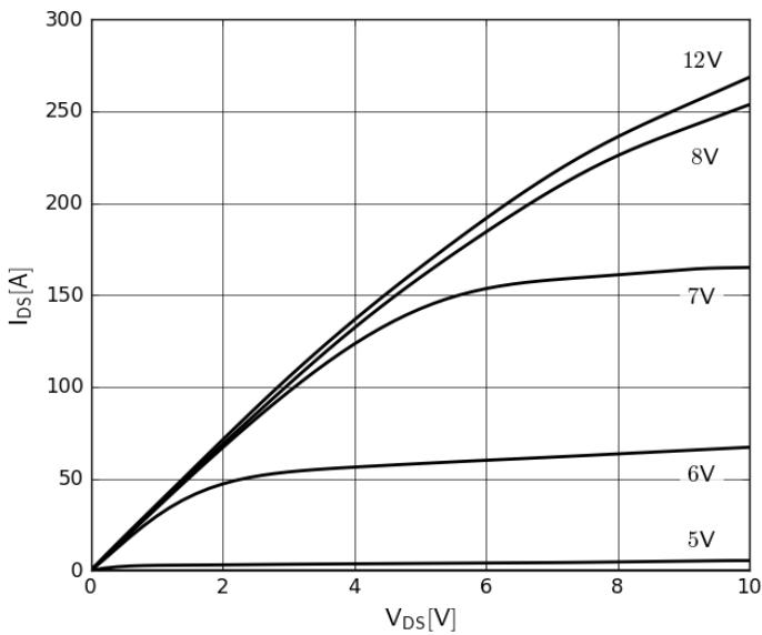
**Figure 1. Typical Output Characteristics  $T_J=25^\circ\text{C}$**
