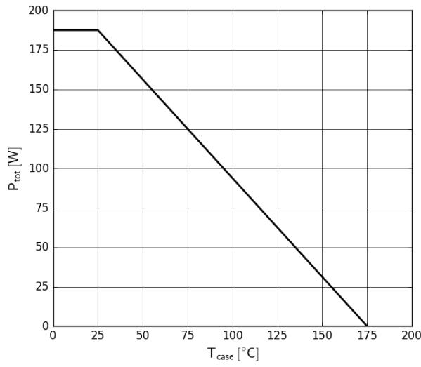
**Figure 9. Power Dissipation**
