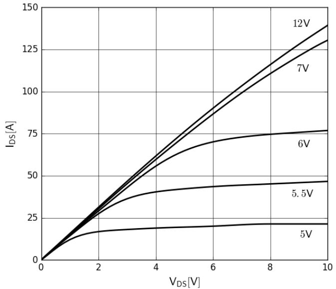
**Figure 2. Typical Output Characteristics  $T_J=175^\circ\text{C}$**
