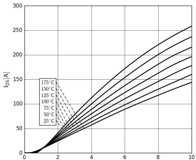
**Figure 8. Forward Characteristics of Rev. Diode**
