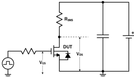
**Figure 17. Dynamic  $R_{DS(on)}$  Test Circuit**
