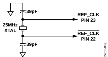
Figure 40. Crystal Configuration for Reference Clock Source
