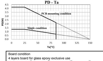
Cu thickness:  $1^{st}$  layer and  $4^{th}$  layer  $55\mu m,\,2^{nd}$  layer and  $3^{rd}$  layer  $35\mu m$
