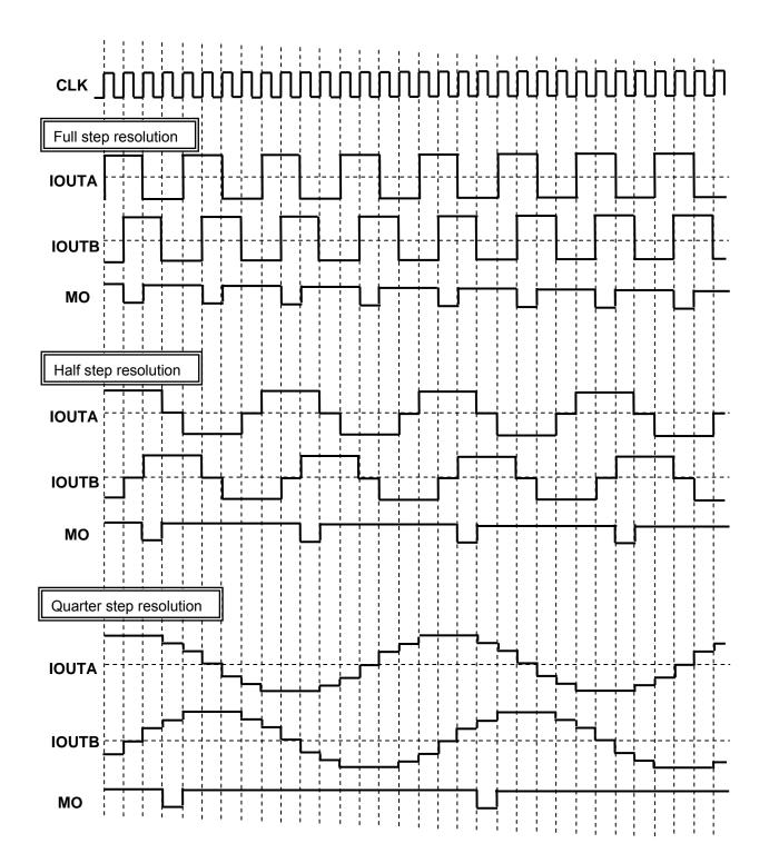
The MO output shown in the timing chart is when the MO pin is pulled-up.
