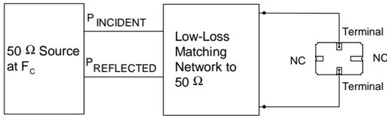
$$CW \text{ RF Power Dissipation} = P_{INCIDENT} - P_{REFLECTED}$$
