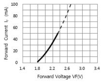
Fig. 2 FORWARD CURRENT VS. FORWARD VOLTAGE
