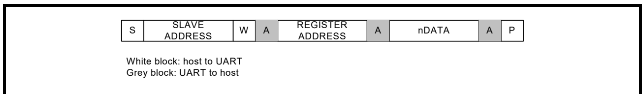
FIGURE 4. MASTER WRITES TO SLAVE (XR20M1170)
