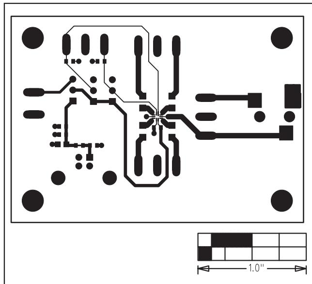
Figure 3. MAX14535E EV Kit PCB Layout—Component Side
