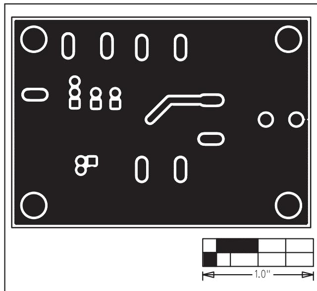
Figure 4. MAX14535E EV Kit PCB Layout—Solder Side
