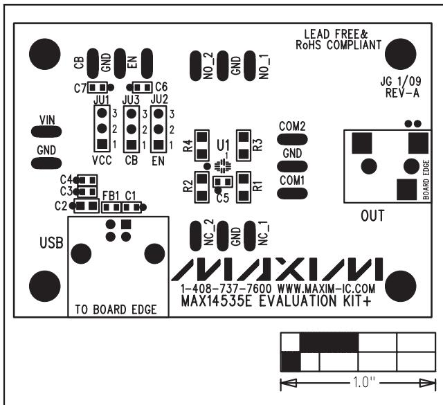
Figure 2. MAX14535E EV Kit Component Placement Guide—Component Side
