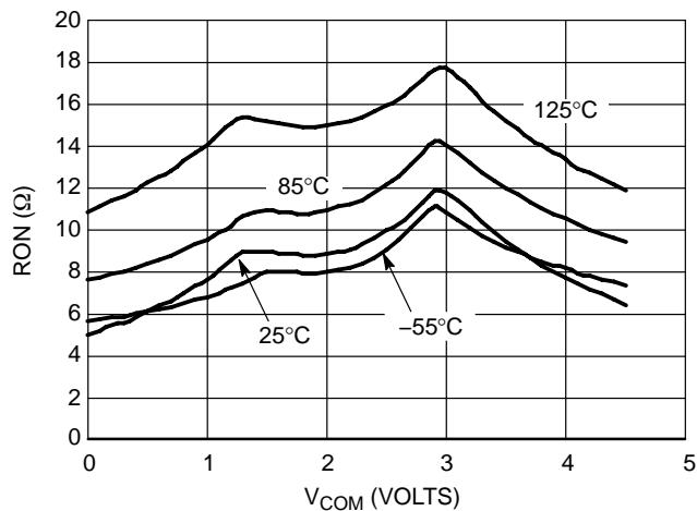
**Figure 21.  $R_{DS(on)}$  versus  $V_{COM}$  and Temperature,
