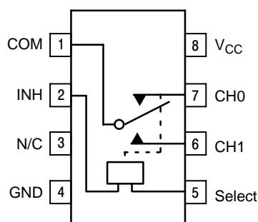
Figure 1. Pin Assignment
