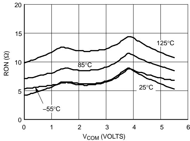
**Figure 23.  $R_{DS(on)}$  versus  $V_{COM}$  and Temperature,
