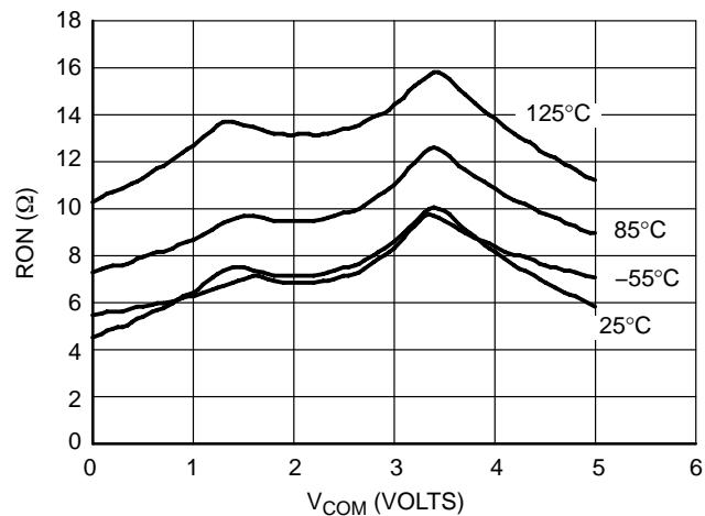
**Figure 22.  $R_{DS(on)}$  versus  $V_{COM}$  and Temperature,
