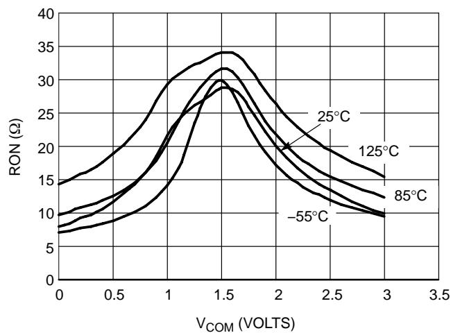
**Figure 20. R<sub>ON</sub> versus V<sub>COM</sub> and Temperature, V<sub>CC</sub> = 3.0 V**
