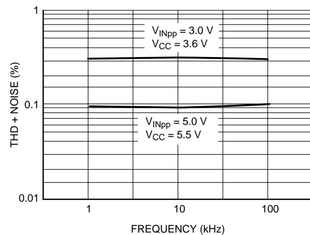
Figure 14. Total Harmonic Distortion Plus Noise versus Frequency
