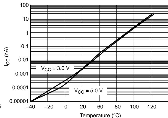
**Figure 16. I<sub>CC</sub> versus Temp, V<sub>CC</sub> = 3 V & 5 V**
