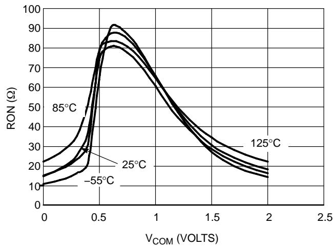
**Figure 18. R<sub>ON</sub> versus V<sub>COM</sub> and Temperature, V<sub>CC</sub> 2.0 V**
