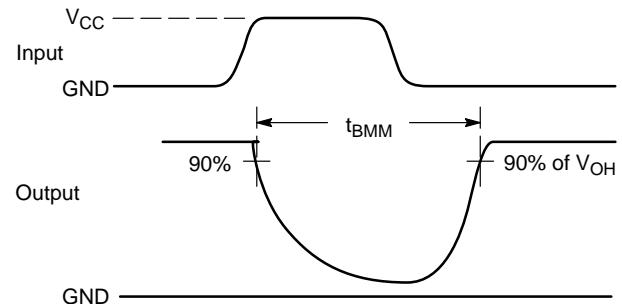
**Figure 3.  $t_{BBM}$  (Time Break-Before-Make)**
