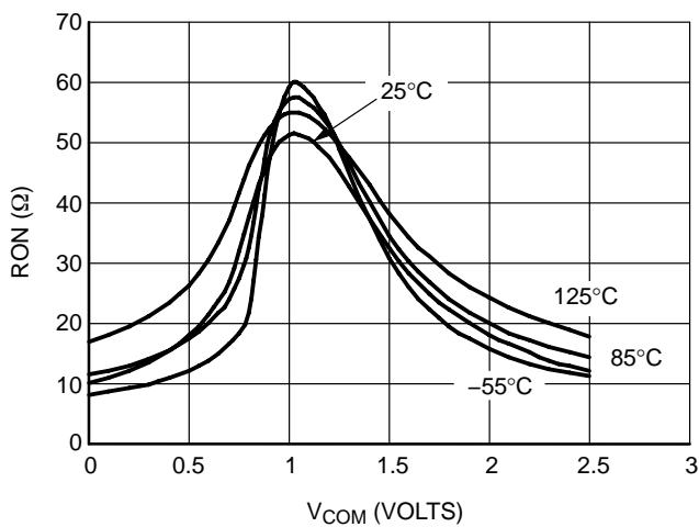
**Figure 19. R<sub>ON</sub> versus V<sub>COM</sub> and Temperature, V<sub>CC</sub> = 2.5 V**
