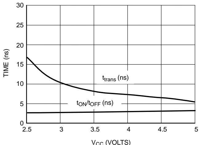
Figure 12.  $t_{ON}$  and  $t_{OFF}$  versus  $V_{CC}$  at  $25^\circ\text{C}$
