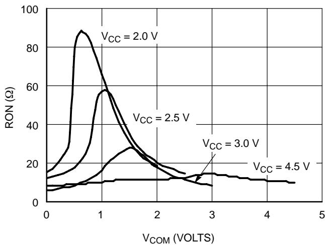
**Figure 17. R<sub>ON</sub> versus V<sub>COM</sub> and V<sub>CC</sub> (@ 25°C)**
