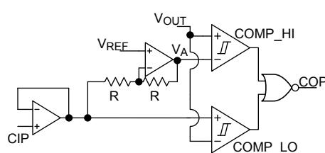
*Figure 2. Internal Window Comparator*
