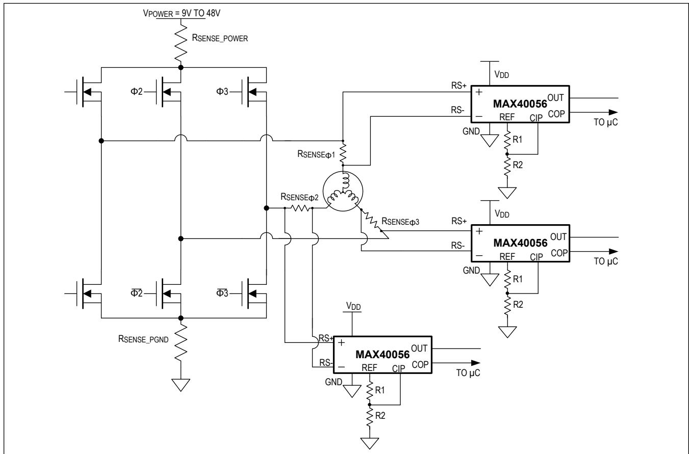
Figure 5. In-Line Current Sensing in Motor Control
