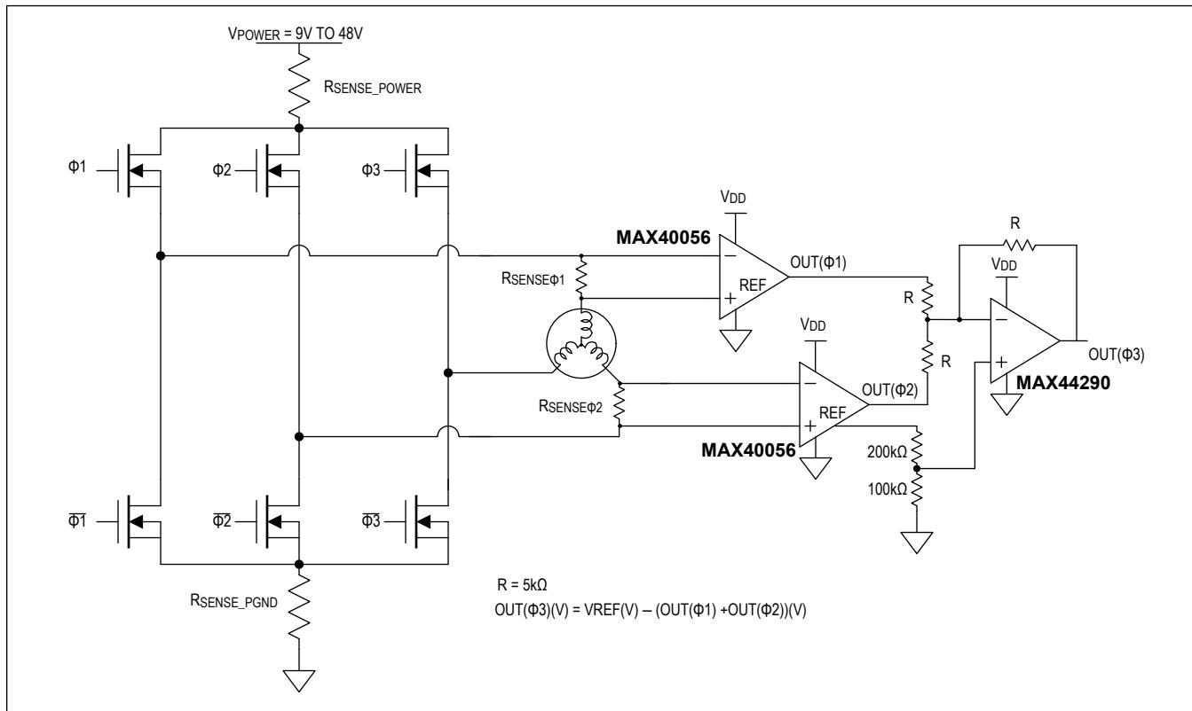
Figure 6. Current Sensing in a 3-Phase Servo Motor
