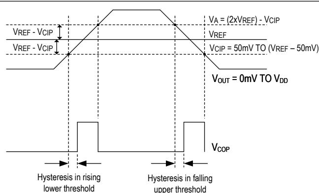
*Figure 3. Window Comparator Hysteresis Waveform*
