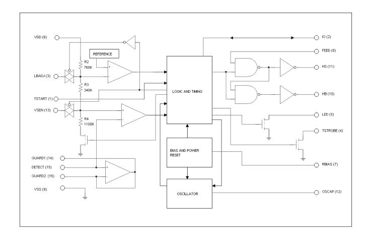
CMOS Ionization Smoke Detector ASIC with Interconnect and Timer Mode Product Specification
