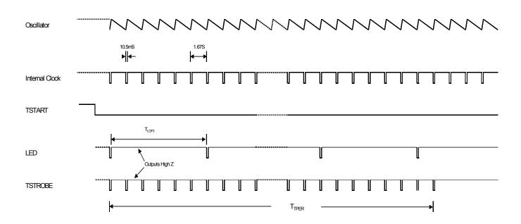
CMOS Ionization Smoke Detector ASIC with Interconnect and Timer Mode
