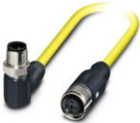
Sensor/Actuator cable, 4-position, PVC, shielded, Plug angled M12-SPEEDCON, A-coded, on Socket straight M12-SPEEDCON, A-coded, Cable length: 0.5 m
