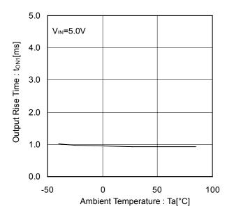
Figure 18. Output Rise Time vs Ambient Temperature
