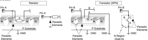
Figure 39. Example of monolithic IC structure
