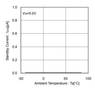
Figure 6. Standby Current vs Ambient Temperature (EN Disable)
