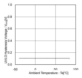
Figure 16. UVLO Hysteresis Voltage vs Ambient Temperature
