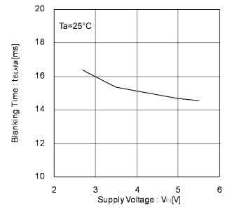
Figure 25. Blanking Time vs Supply Voltage
