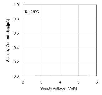
Figure 5. Standby Current vs Supply Voltage (EN Disable)
