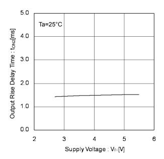
Figure 19. Output Rise Delay Time vs Supply Voltage
