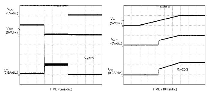
Figure 33. Over-Current Response Output Short Circuit at Enable
