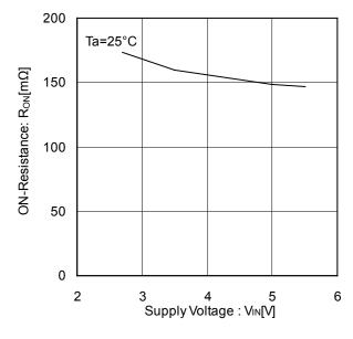
Figure 9. ON-Resistance vs Supply Voltage
