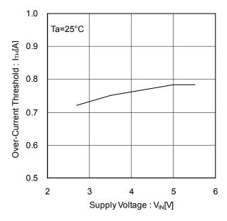
Figure 11. Over-Current Threshold vs Supply Voltage
