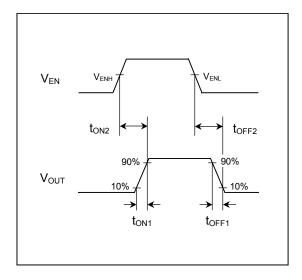
Figure 2. Timing Chart at Output Rise / Fall Time
