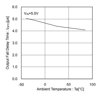
Figure 24. Output Fall Delay Time vs Ambient Temperature
