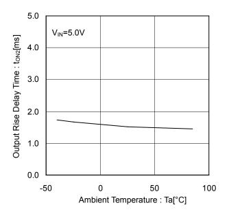
Figure 20. Output Rise Delay Time vs Ambient Temperature
