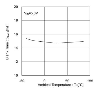
Figure 26. Blank Time vs Ambient Temperature
