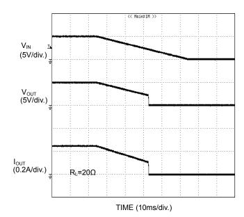
Figure 35. UVLO response  $V_{\text{IN}}$  Decreasing
