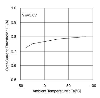
Figure 12. Over-Current Threshold vs Ambient Temperature
