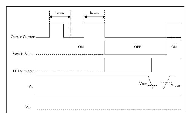
Figure 37. Over-Current Shutdown Operation (Reset at reclosing of power supply V<sub>IN</sub>)
