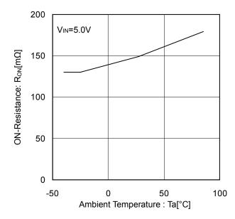
Figure 10. ON-Resistance vs Ambient Temperature
