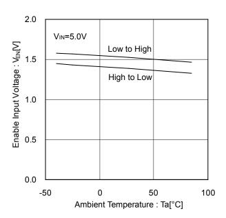
Figure 8. EN Input Voltage vs Ambient Temperature
