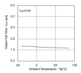
Figure 22. Output Fall Time vs Ambient Temperature
