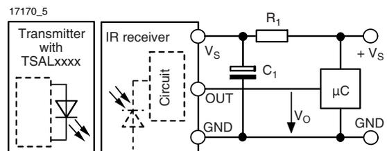
$R_1$  and  $C_1$  are recommended for protection against EOS. Components should be in the range of  $33 \Omega < R_1 < 1 \text{ k}\Omega$ ,  $C_1 > 0.1 \mu\text{F}$ .
