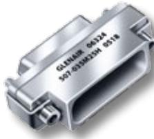
**Potting Shells** provide easy encapsulation of Micro-D solder cup terminations. These potting shells provide .25 inches (6.3 mm.) of depth.
