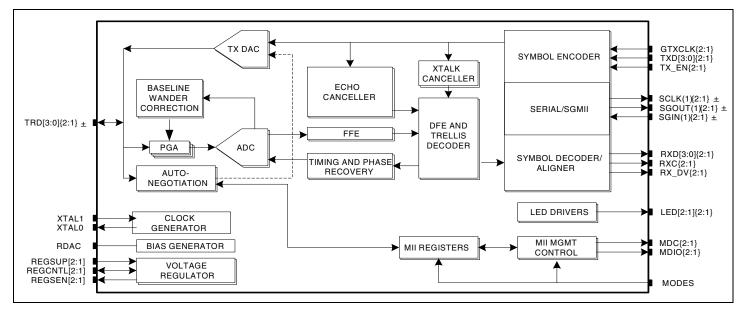
A member of Broadcom's third generation of Gigabit Ethernet PHYs, the **BCM5482** consists of two complete 10/100/1000BASE-T Gigabit Ethernet transceivers integrated on a single monolithic CMOS chip. The **BCM5482** is optimized for low power and small footprint size to reduce design complexity for space-constrained IP phone applications. For 10/100BASE-TX applications, the single package offers a compelling advantage over two single devices for Gigabit uplinks.
