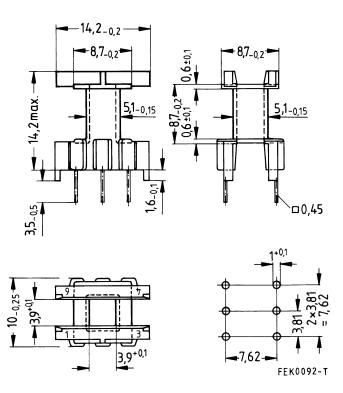
Hole arrangement View in mounting direction
