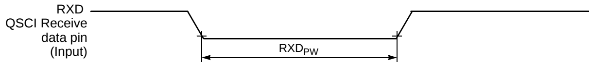
Figure 10-12 RXD Pulse Width
