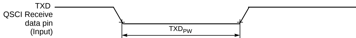
Figure 10-13 TXD Pulse Width
