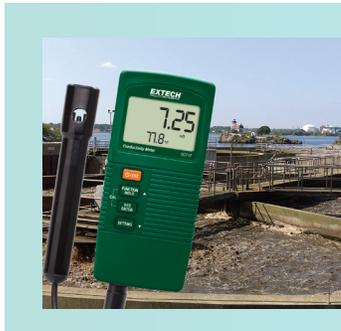
**Compact handheld Conductivity Meter with long life carbon rod combination electrode measures Conductivity, TDS and Temperature. Units of measure include  $\mu\text{S}/\text{cm}$ ,  $\text{mS}/\text{cm}$ ,  $\text{ppm}$ ,  $^{\circ}\text{F}$ , and  $^{\circ}\text{C}$ . The meter features three ranges for Conductivity and TDS plus adjustable Temperature compensation factor to maintain accuracy.**
