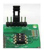
Set the Mode Switch to Mode1 (as above) and place a jumper between Pin3 and Pin4 of the PICkit programming connector (as shown in the picture) before power up or reset.
