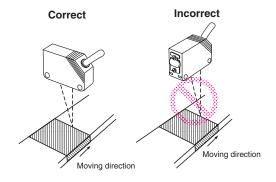
The stability indicator may turn off in reaction to reflection from background objects. In such cases, incline the Sensor by 10° as shown in the illustration for more stable detection.
