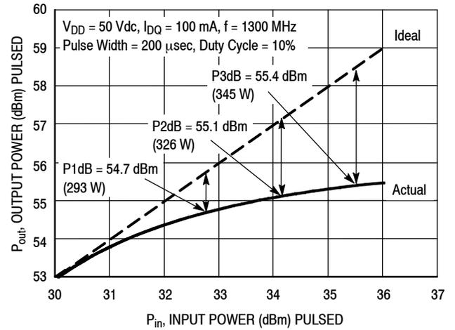
**Figure 4. Pulsed Output Power versus Input Power**
