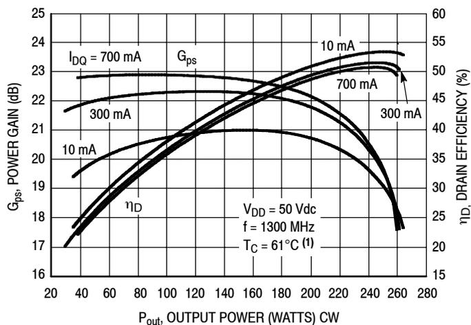
1. Data for graph was collected in a water cooled test fixture. The water inlet temperature = 25°C.
