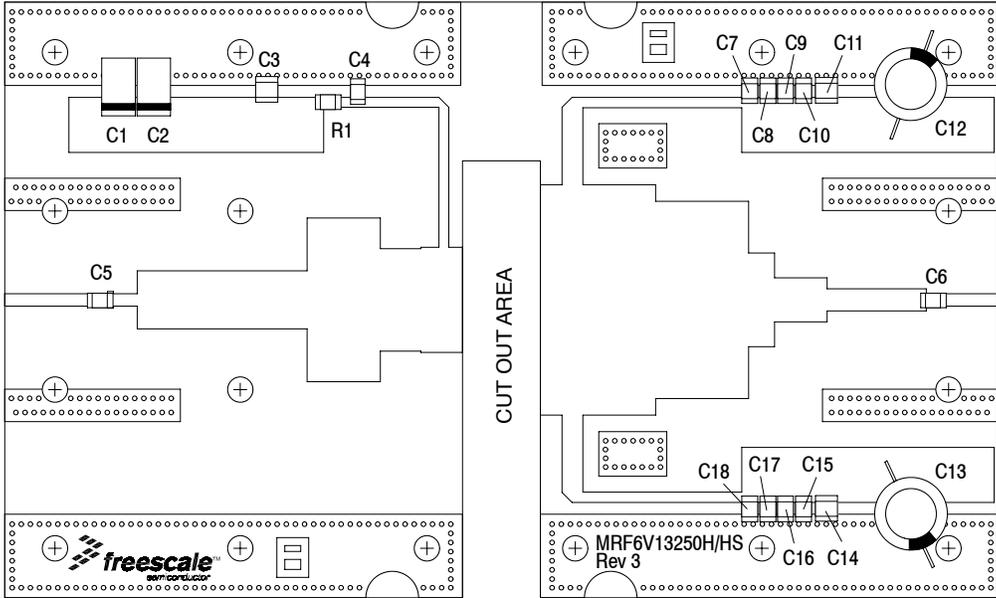
Figure 2. MRF6V13250HR3(HSR3) Test Circuit Component Layout — 1300 MHz
