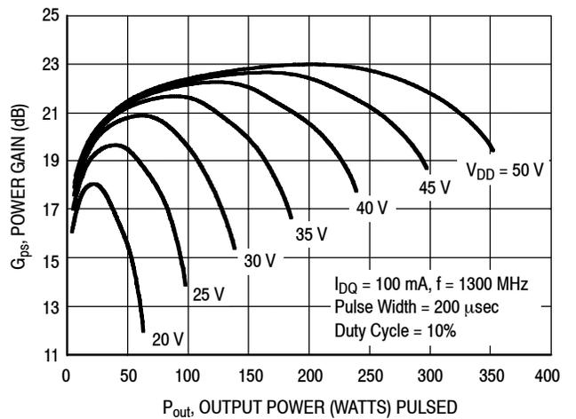
**Figure 6. Pulsed Power Gain versus Output Power**
